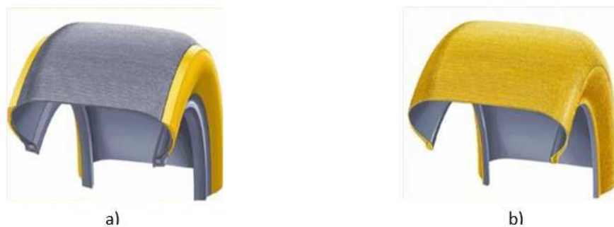
Figure 2 a) sidewall b) carcass[4]
