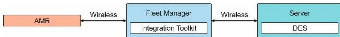
Figure 3 Communication schema between DT and AMR vehicle
