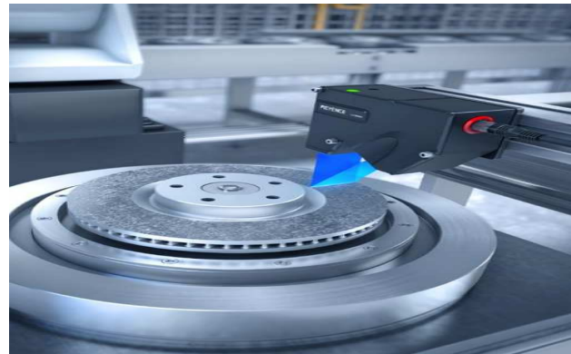
Figure 2 Measurement process with profilometer [7]
