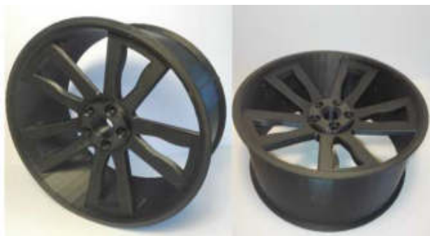
Figure 10 Physical model made by 3D printing
