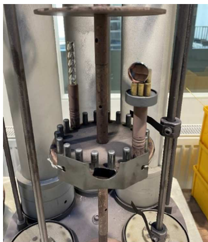
Figure 3 Samples in the preparation in a vacuum chamber
