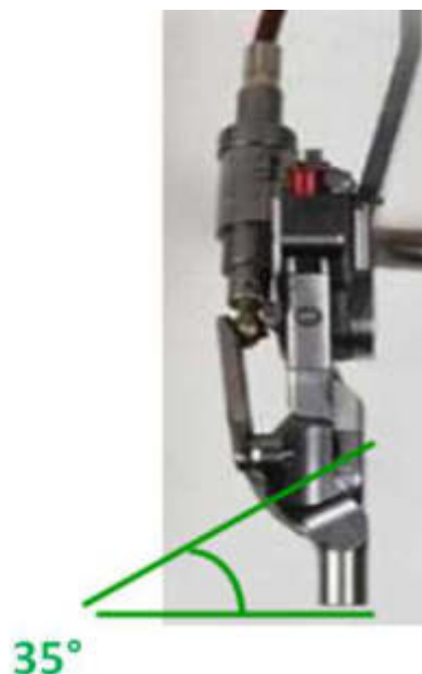
Figure 4 Axis joint with 35 ° inclination
